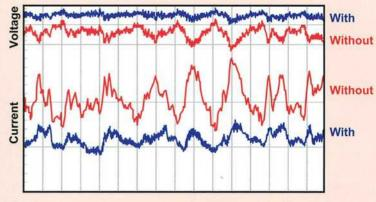
free switching to eliminate spikes that are typically associated with conventional electromechanical switching.
