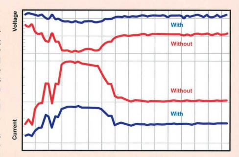
protection against voltage drops in the networks, eliminating load peaks and higher utilization of equipment through obtaining maximum torque during start-ups.
