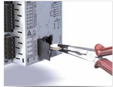
Abb.: Replacing the battery using long-nose pliers
