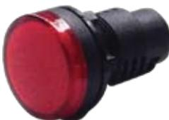
Ø30   | AD16-30 D/S   | <ul style="list-style-type: none"> <li>Rated Voltage: AC/DC: 6V, 12V, 24V, 36V, 48V, 110V</li> <li>AC: 220V, 380V</li> <li>DC: 220V</li> <li>Mounting Hole: 30mm</li> </ul> |
