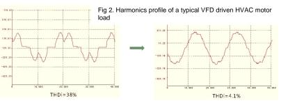
Fig 3. Harmonics current waveform distortion seen on typical 6-pulse VFD load before and after harmonics filtering
