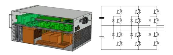
Fig 5. AHF and SVG are IGBT technology product designed to solve harmonics and PF swing problem in critical facility
